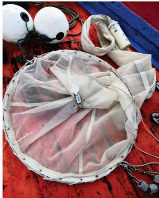
Figure 2: A larvae net with a one meter diameter circular frame and 500 micron mesh net was used to sample the spiny lobster phyllosoma
